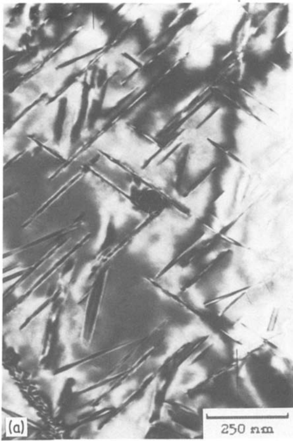
Figure 5 Bright field/dark field pair of the 1.0% Li-4.5% Cu alloy aged for 128 h; (a) bright field image; (b) corresponding \beta'/\theta' dark field image.
